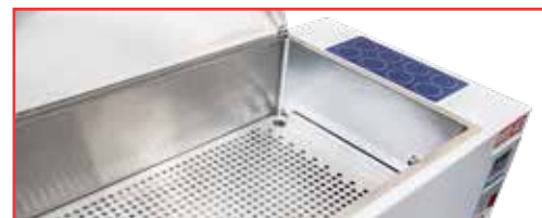
Bottom stainless steel holed platform and plastified stand
