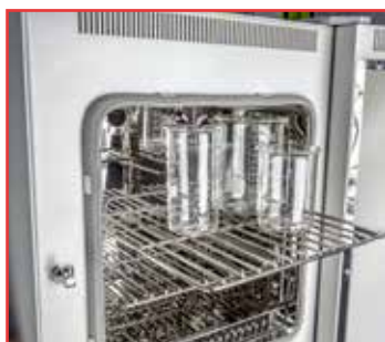
Wire shelves with no overturning system to always operate safely
