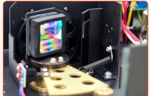
Monochromator: grating with 1200 lines/mm
